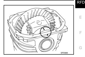
6. Install side oil seal. Refer to RFD-9, "Removal and Installation".
