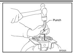
5. Remove the pinion mate shaft.
