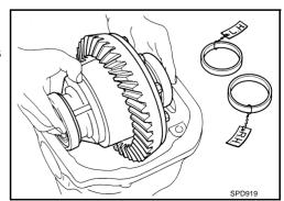
Insert original left and right side bearing adjusting washers in place between side bearings and carrier.
