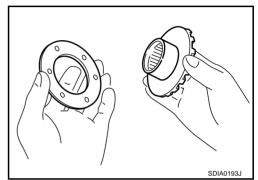
3. Install the side gears, thrust washers, pinion mate gears, thrust washers into differential case.
