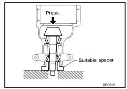
6. Install front oil seal with tool. Refer to RFD-7, "Removal and Installation".
