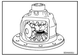
7. Check mating surfaces of differential case, side gears, pinion mate gears, pinion mate shaft and thrust washers.
