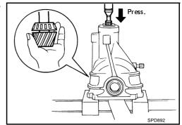
8. Remove pinion bearing outer races with a brass drift.
