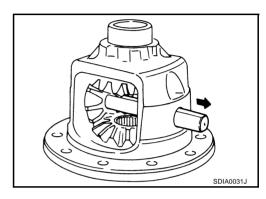
6. Turn the pinion mate gear, then remove the pinion mate gear, pinion mate thrust washer, side gear and side gear thrust washer from the differential case.
