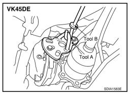
Remove side oil seal using a flat-bladed screwdriver.
