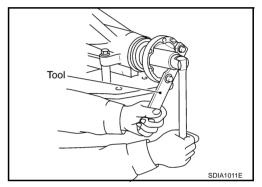
8. Tighten the drive pinion lock nut by very small degrees until the specified preload in achieved, when checking the preload, turn drive pinion in both directions several times.
