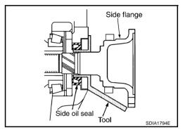
c. Put suitable drift on the center of side flange, then drive it until sound changes.
