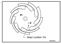
There are two numbers painted on the drive pinion. The first one refers to the drive pinion and drive gear as a matched set. This number should be the same as the number on the drive gear. The second number is the "pinion head height number". It refers to the ideal pinion height from standard for quietest operation. Use the following chart to determine the correct pinion height washer.
