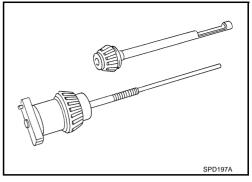
3. Install the pinion rear bearing inner race into the final drive housing. Then place the pinion preload shim selector tool, J34309-1, gauge screw assembly.
