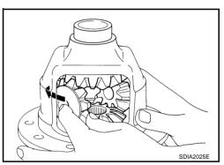
4. Fit pinion mate shaft to differential case so that it meets lock pin holes.
