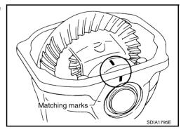
6. Measure the turning torque of the carrier at the drive gear retaining bolts with a spring gauge, J-8129.
