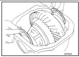
Align matching mark on bearing cap with that on gear carrier.
