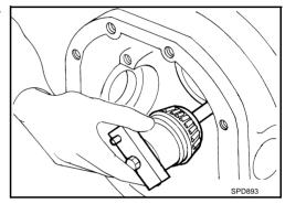
4. Assemble the pinion front bearing inner race and the J34309-2 gauge anvil. Assemble them together with the J34309-1 gauge screw in the final drive housing. Make sure that the pinion height gauge plate, J34309-16, will turn a full 360 degrees. Tighten the two sections together by hand.
