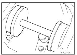
2. Select the correct standard pinion height adjusting washer thickness. Select by using a standard gauge of 3 mm (0.12 in) and your J34309-101 feeler gauge. Measure the distance between the J34309-11 pinion height adapter including the standard gauge and the arbor.
