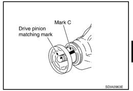
3. Using the drive pinion flange wrench, remove drive pinion lock nut.
