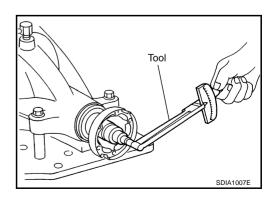
When checking preload, turn drive pinion in both directions several times to seat bearing rollers correctly.
