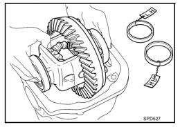
3. Insert left and right original side bearing adjusting washers in place between side bearings and carrier.
