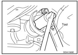
5. Remove front oil seal using the side bearing outer race puller,
